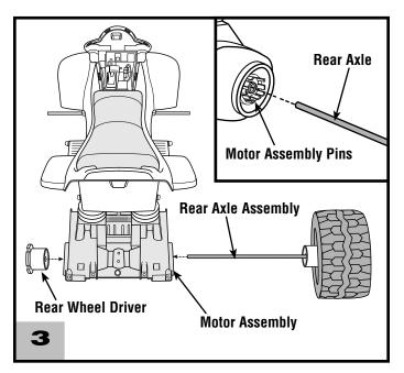
• Position the vehicle upright. Face the back end of the vehicle. *Hint:* You will need to temporarily hold the remaining rear wheel driver onto the motor assembly to properly position the rear axle assembly into the motor assembly.
